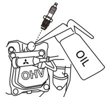
4. Replace the spark plug and pull starter handle until resistance is felt.
